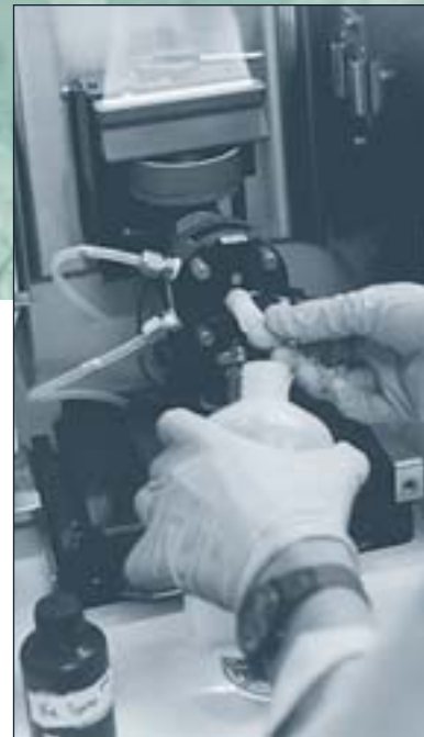
Students use instrumentation such as a flame atomic absorption spectrophotometer.
